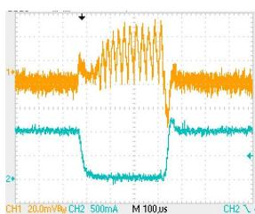
Buck Load Transient Response (Ibuck=10mA to 200mA, VBAT=3.6V, Vbuck=1.2V,Cout=4.7uF)
