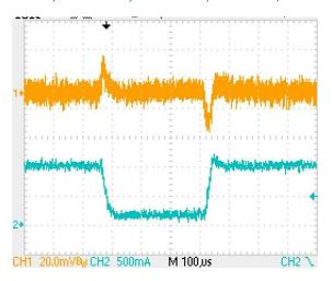
Buck No Load Output Voltage Ripple (VBAT=3.6V, Vbuck=1.2V,Cout=4.7uF)
