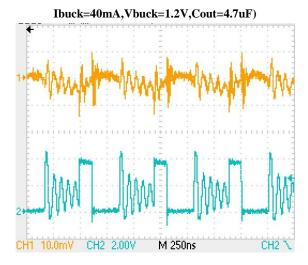
Buck Output Voltage Ripple Vs LX (VBAT=3.6V,
