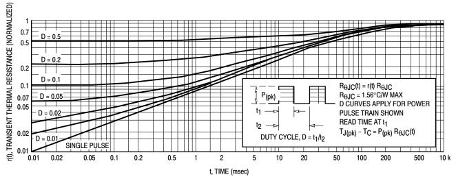
Figure 9. Typical Thermal Response for MJE13007
