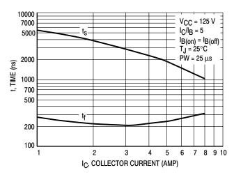
Figure 11. Turn-Off Time (Resistive Load)
