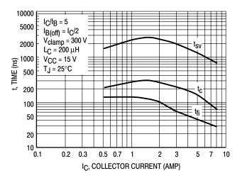
Figure 13. Typical Inductive Switching Times
