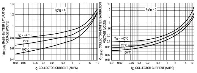
Figure 1. Base-Emitter Saturation Voltage
