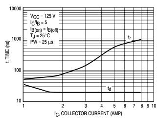
Figure 10. Turn-On Time (Resistive Load)
