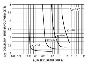
Figure 3. Collector Saturation Region
