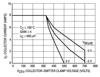
Figure 7. Maximum Reverse Bias Switching Safe Operating Area
