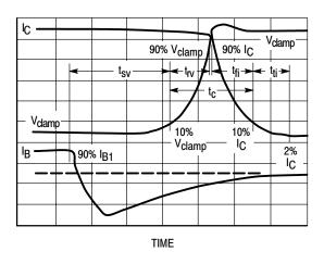
Figure 12. Inductive Switching Measurements
