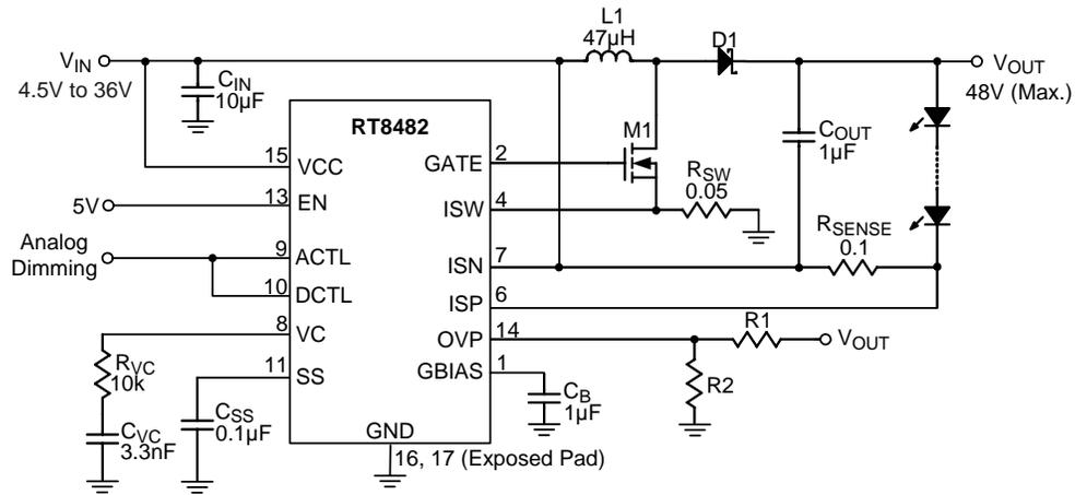
Figure 3. Analog Dimming in Buck-Boost Configuration
