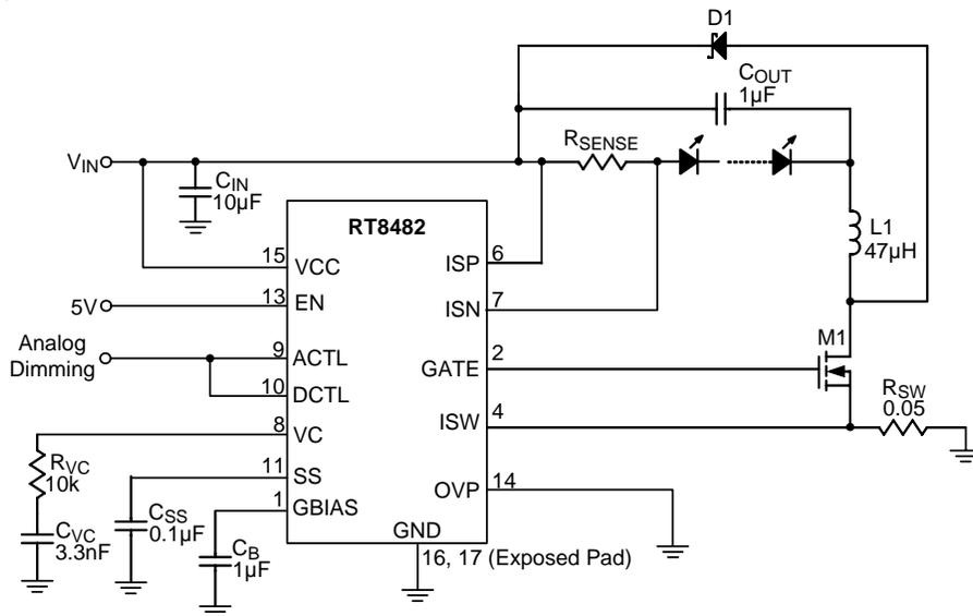
Figure 4. Analog Dimming in Buck Configuration
