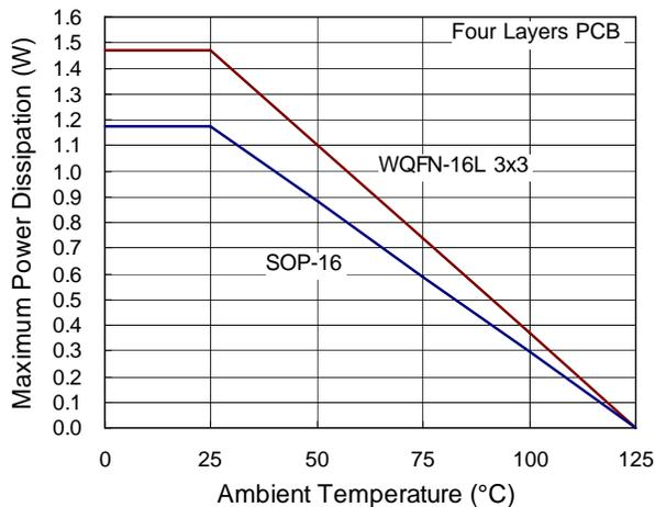
Figure 5. Derating Curves for RT8482 Packages
