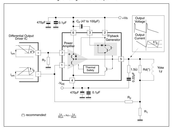
Figure 7: Using a Differential-output Driver
