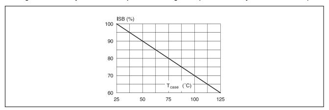
Figure 9: Secondary Breakdown Temperature Derating Curve (ISB = Secondary Breakdown Current)
