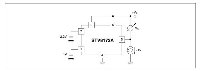
Figure 3: Measurement of  $\rm V_{3L}$  and  $\rm V_{5L}$
