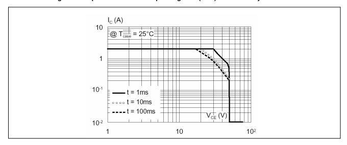
The diagram has been arbitrarily limited to max I0 (2 A).
