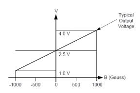
obtained with a supply voltage of 5V, but at the cost of increased supply current and a slight loss of output symmetry. So, it is not recommended to work in such condition unless the output voltage magnitude is a main issue. The output signal can be capacitively coupled to an amplifier for boosting further if the changing frequency of the magnetic field is high.
