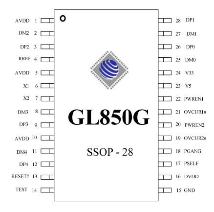
Figure 3.2 – GL850G 28 Pin SSOP Pinout Diagram
