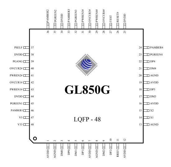
Figure 3.1 – GL850G 48 Pin LQFP Pinout Diagram
