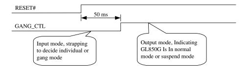
Figure 5.5 – Timing of PGANG/SUSPEND strapping
