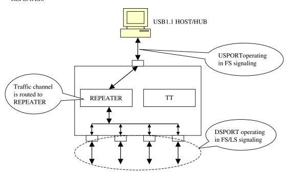
Figure 5.1 – Operating in USB 1.1 scheme
