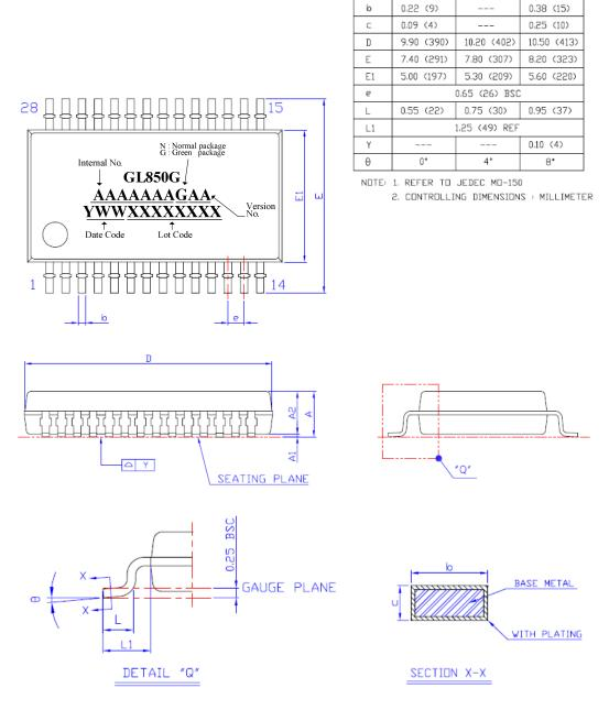
Figure 7.2 - GL850G 28 Pin SSOP Package
