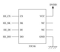
Figure 5.9 - Schematics Between GL850G and 93C46
