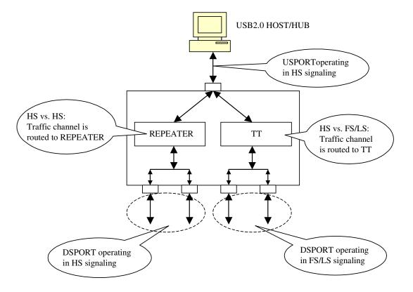
Figure 5.2 – Operating in USB 2.0 scheme
